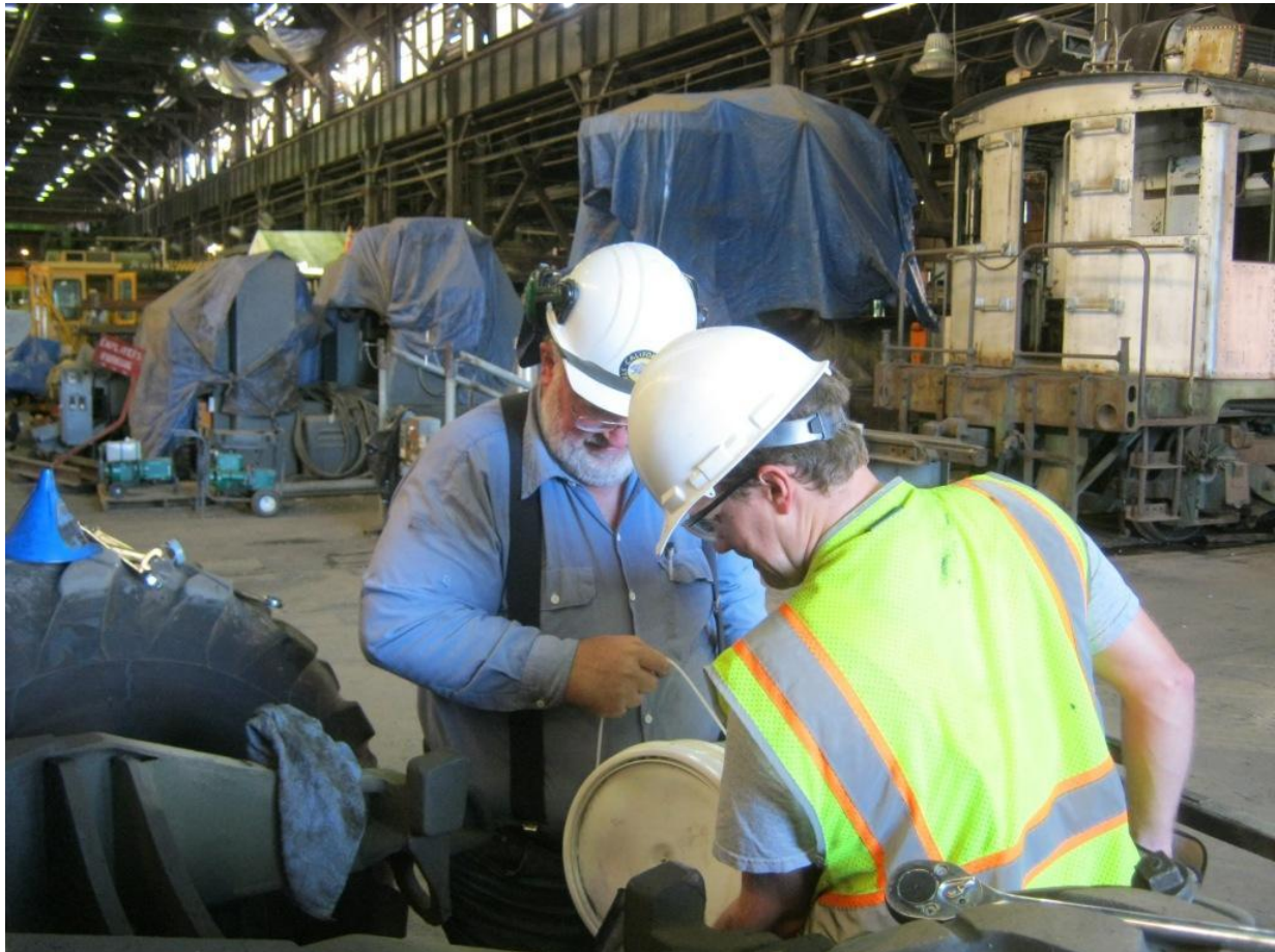
Frank and DJ replace the differential oil in the Green Machine
