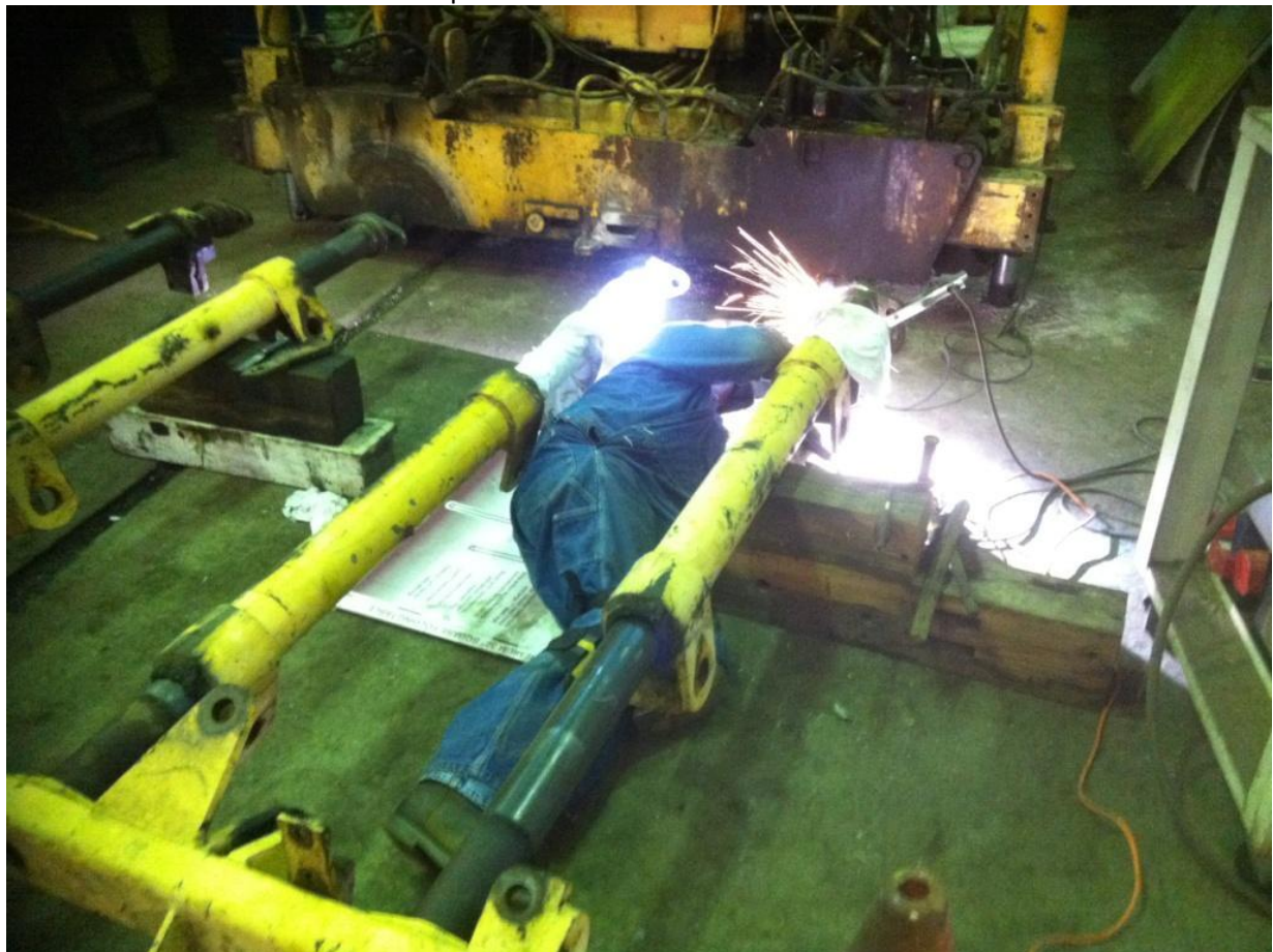
Cliff welds cracks in the slide mounts
